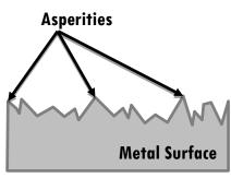
both the tool and workpiece, it is important to understand that a metal surface, although appearing to be smooth to the naked eye, is not. The surface actually contains asperities as seen the in this picture.
