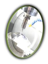
Oil based metalworking fluids, otherwise known as straight oils, are meant to be used in tough operations where lubrication and extreme pressure properties are necessary.
