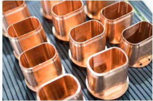
Copper tube scrap parts due to an inconsistent finish. Copper is a more gummy metal and synthetics do not provide the same finish consistency when machining as hybrid semi-synthetics do.
