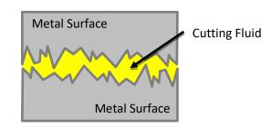
additives are very important for protection, providing a cushion between the two surfaces by filling in around the asperities.
