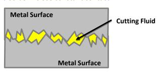
The local temperature at the point of cut can reach up to ~1,000 °C, which can cause the two surfaces to "weld" together. However, when extreme pressure additives are "activated," they react with the surface of each metal to create a low shear strength film that prevents welding.
