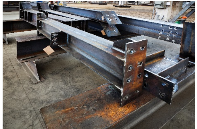
Unprotected Rusted Beam
